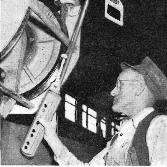
PUSH-BUTTON CRANE: Crane Floorman A. H. Dixon operating one of the new travelling cranes at Newport 'Shops.
