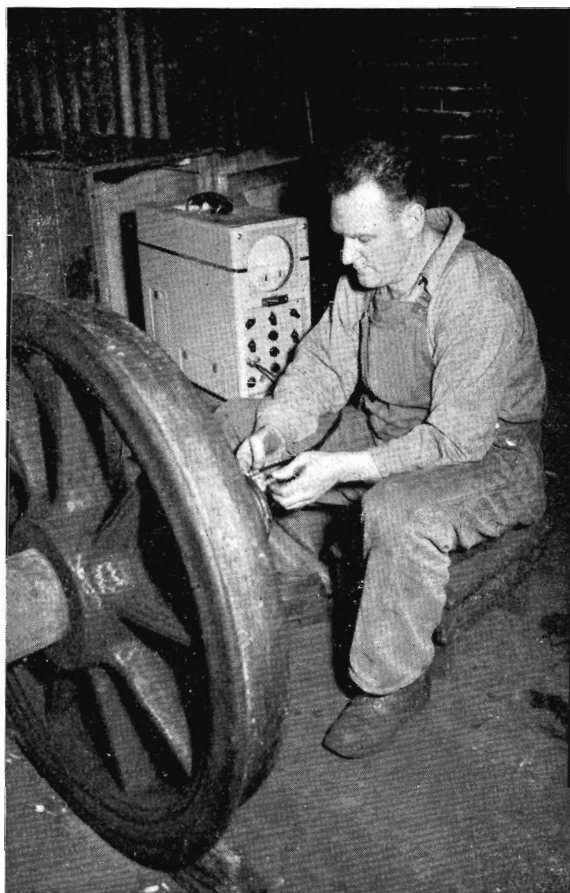
Fitter H. Clancy, Newport Workshops, applies the probes to an axle to be tested.
