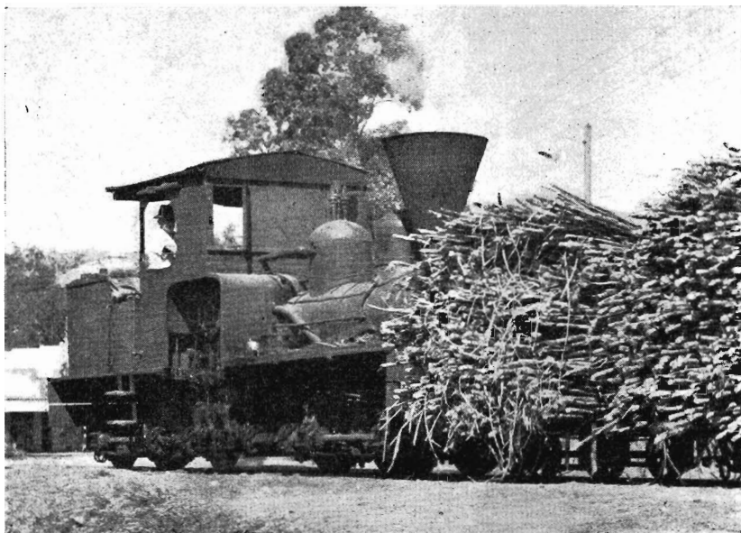
Last remaining Shay geared locomotive in Australia is this one, operated by the Nambour Sugar Mill, Queensland, on its extensive 2 ft. gauge tramway. Note the offset boiler and the vertical cylinders driving each axle through a longitudinal shaft and bevel gears. Photo: A. R. Lyell
