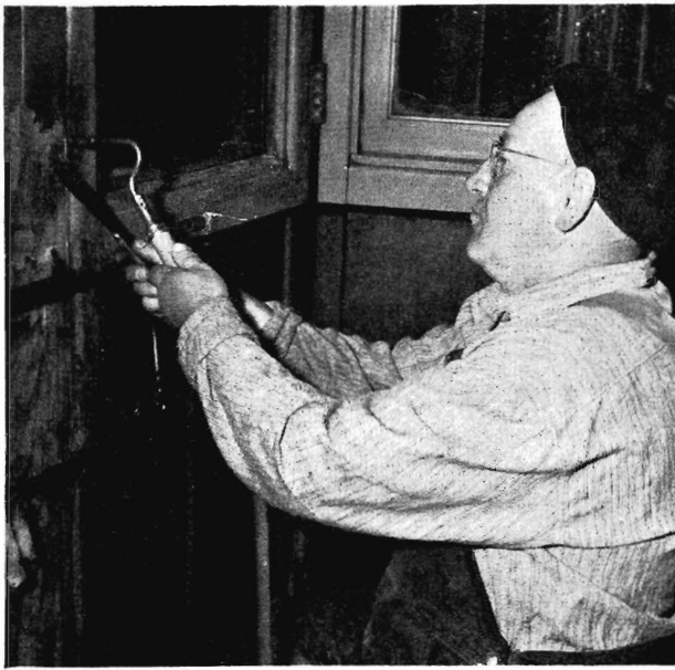
(Above) Painter's Labourer D. Brankovic using an acetylene torch, in place of the old blow-lamp, to remove exterior paint. Car Builder J. Lackner scrapes down a seat back to restore the natural wood colour.
