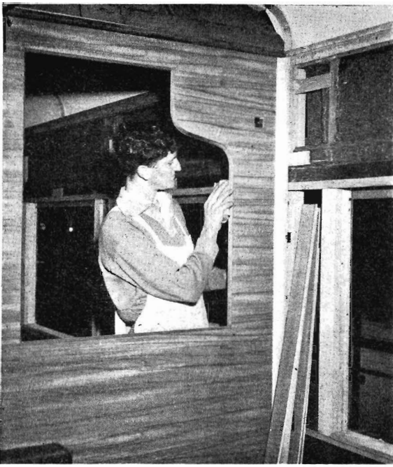
Car Builder J. Bell fitting moulds to the cross partition. Selected and matched walnut veneers are used throughout the car. A section of the hair felt that insulates against noise can be seen on the upper right.
