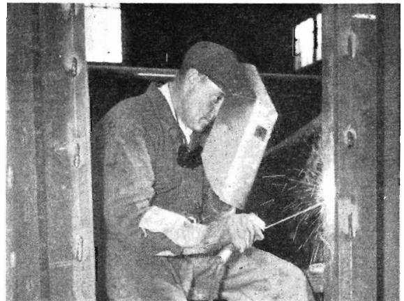
Boilermaker C. Britt at work on the end doorway of car 2 BZ.
