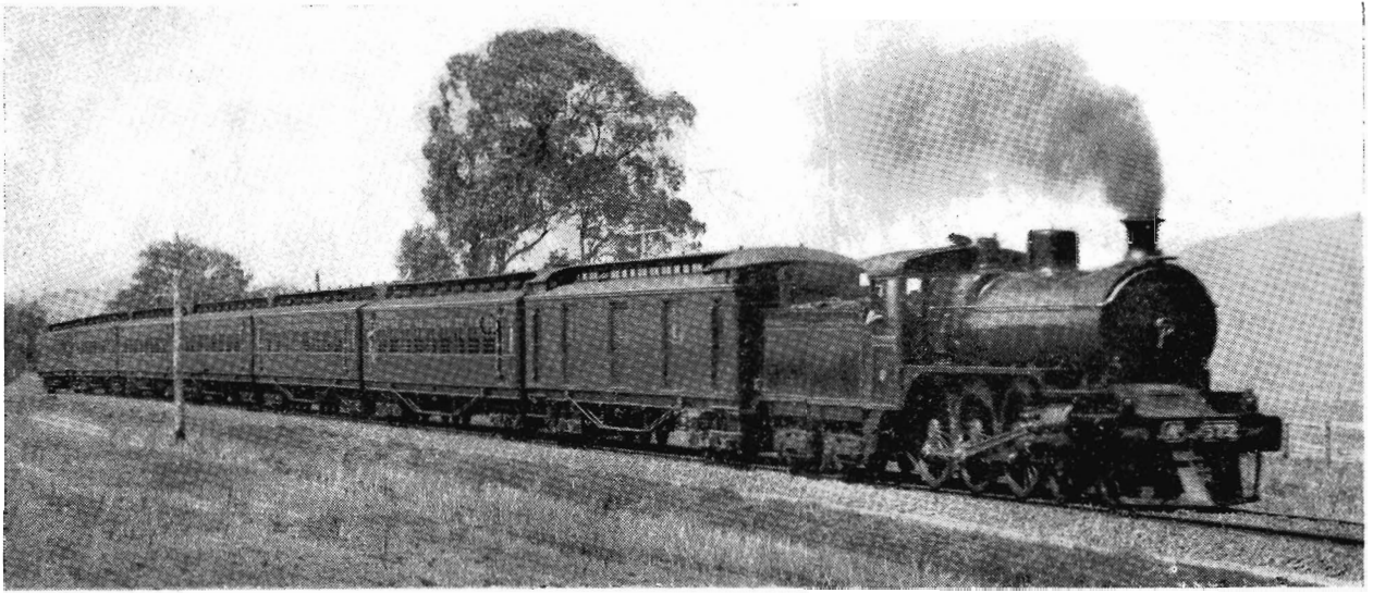
A2 572 hauling the Sydney Express of 1908, with its newly introduced AE and BE cars.
