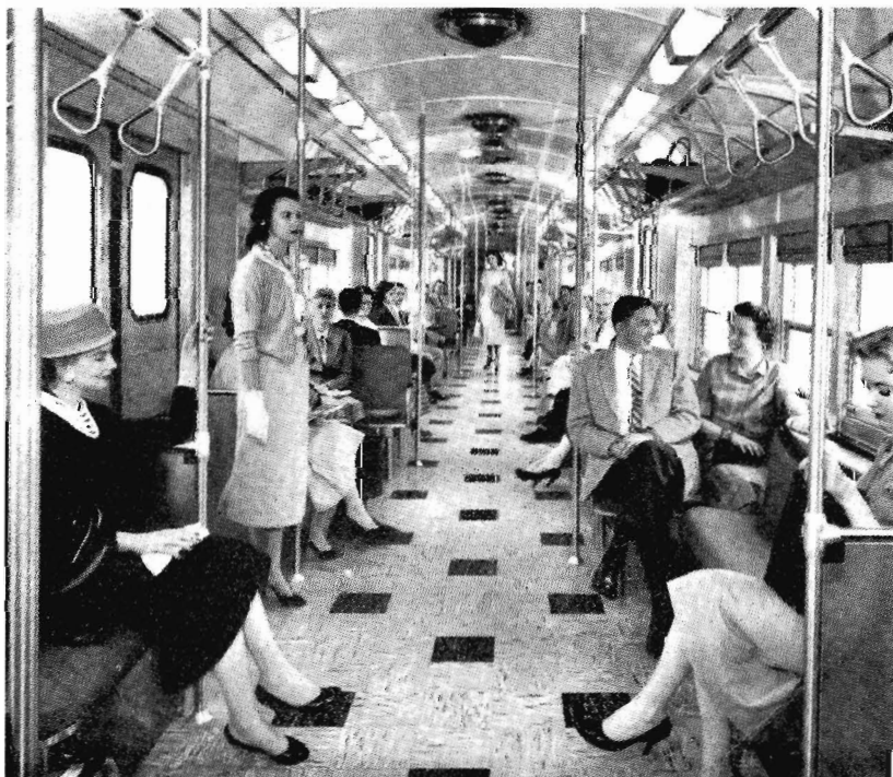
Budd car, specially designed for high-density commuter traffic, is 85 feet long. Built for the Brazilian Railways, the cars will operate in units of three. They are electrically powered, and have four doors to a side, for quick entrance and exit. Seating capacity of each car is 80, and there is space for 320 standees. Harris Trains provide for about 65% standing in crush load, as compared with 80% for these Brazilian cars.
