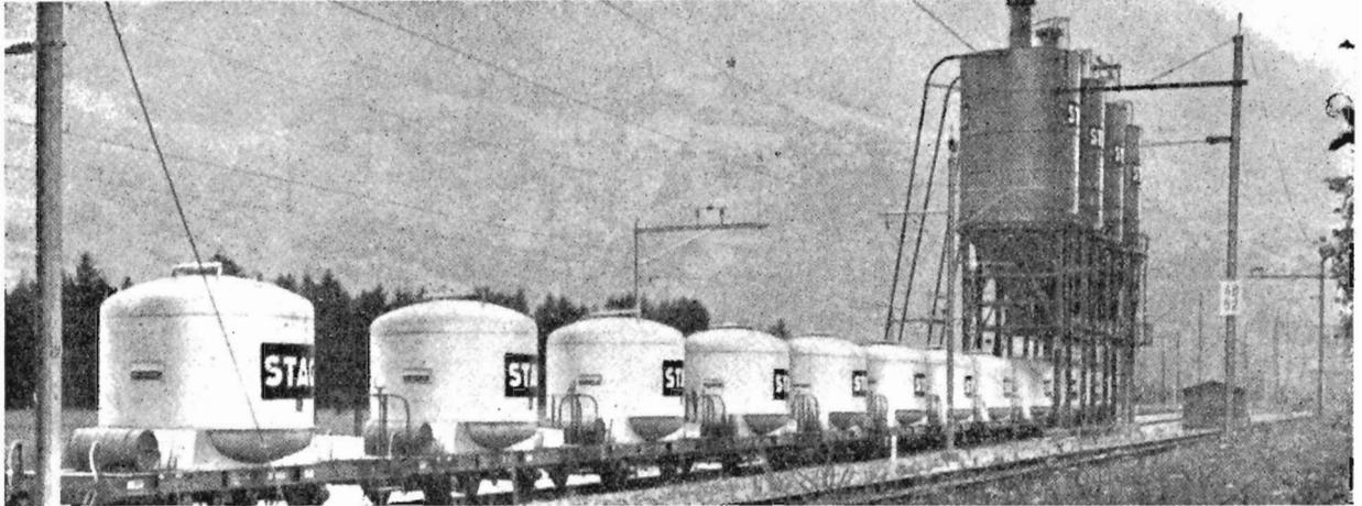
Train of cement containers passing under silo to receive material stored from standard-gauge waggons.
