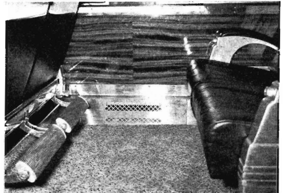
Showing the adjustable footrests, the grill of the electric floor heater and (on the seat arms) the buttons that operate the seat reclining mechanism.
